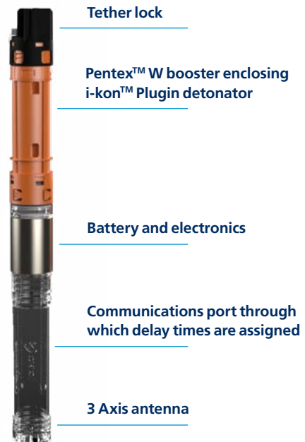
WebGen™ uses low frequency magnetic induction signals to transmit firing commands
